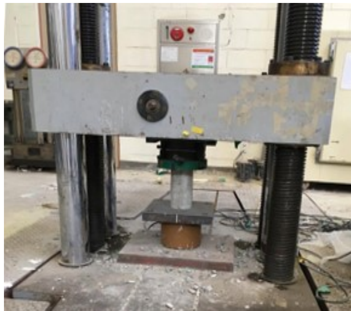
Figure 3-3 Compressive test machine
