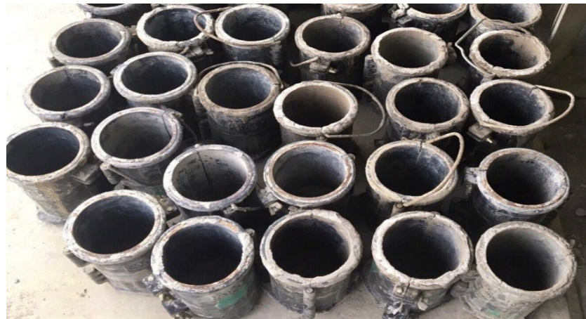
Figure 3-1 Cylindrical shaped mold for casting
