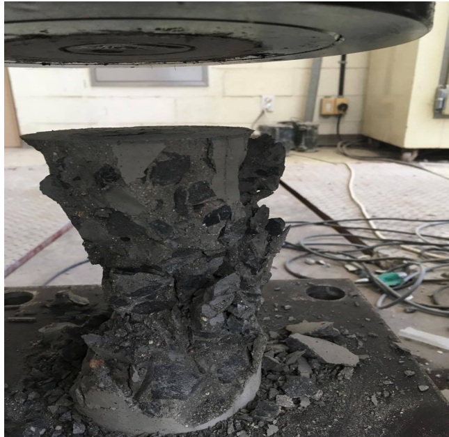
Figure 3-4 Specimen after the compression
