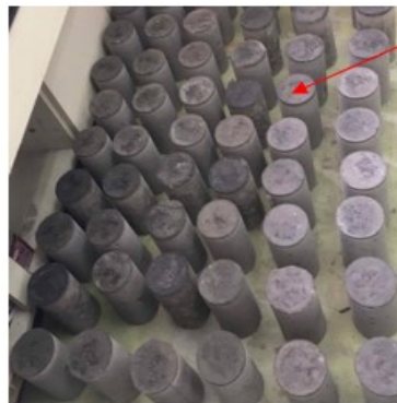
Figure 3-2 Curing the specimen
