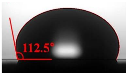
Fig. 3-4. Water contact angle of 18.50 nm Ag on alumina
