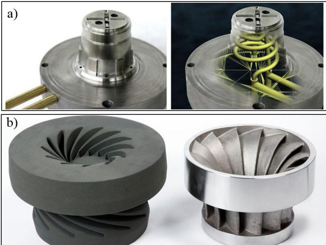
Figure 1.15: (a) An injection mold manufactured by SLM and its vertical cross-section revealing conformal cooling channel, (b) a sand casting mold produced by SLS technique and a casting product (Image source: MODIA, Voxeljet)
