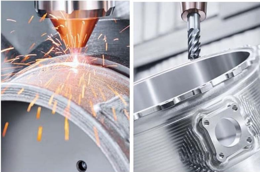
Figure 1.11: Hybrid Additive Manufacturing combined between DED (left) and then CNC process (right) ( Images source: DMG MORI )
