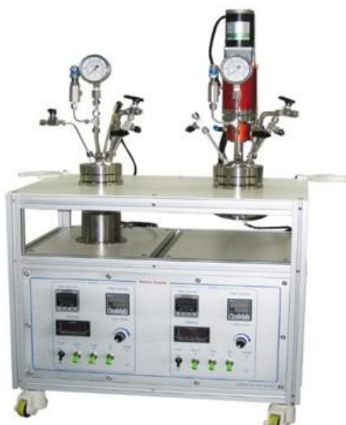
Fig. 2. 6. 100 mL autoclave reactor for hydrogenation of D-glucose.
