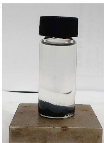
Figure 3. Magnetic nZVI as synthesized in AEERL via chemical reduction method.
