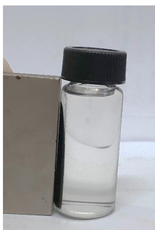
Figure 3. Magnetic nZVI as synthesized in AEERL via chemical reduction method.
