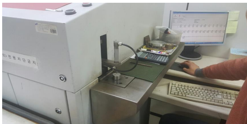
Figure 3.1 Analysis of alloying elements by spark emission spectrometer.
