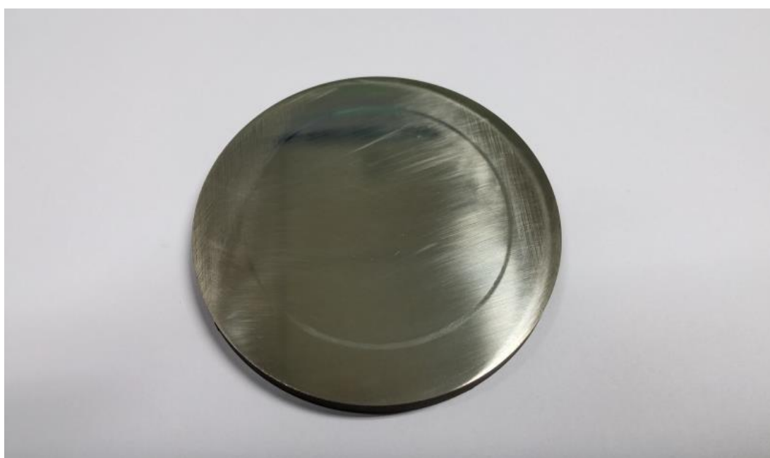
Figure 4.19 Pin on Disk wear test.
