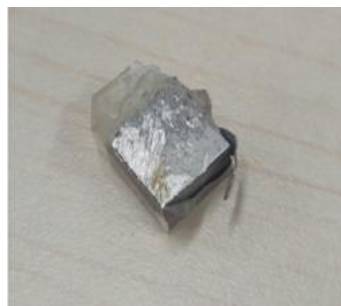
Fig 25. Broken Sample images of the STS316L + Cu powder
