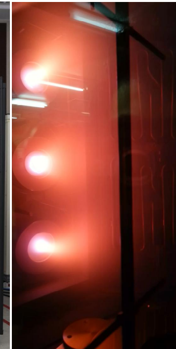
Figure 3-2. Layout inside the chamber (left), photo of arc ion plating equipment(center) and it' s arc plasma during coating process (right)
