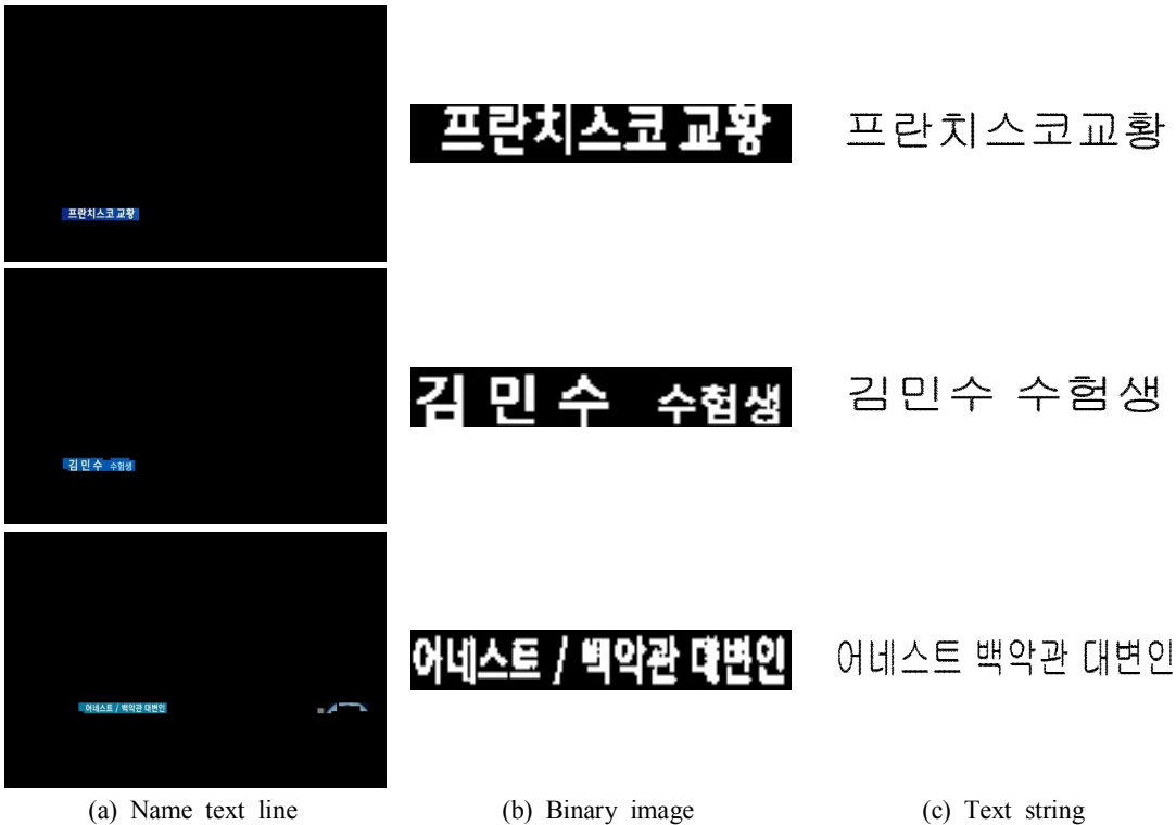
Fig. 6.6. The examples of an experimental result of text recognition
