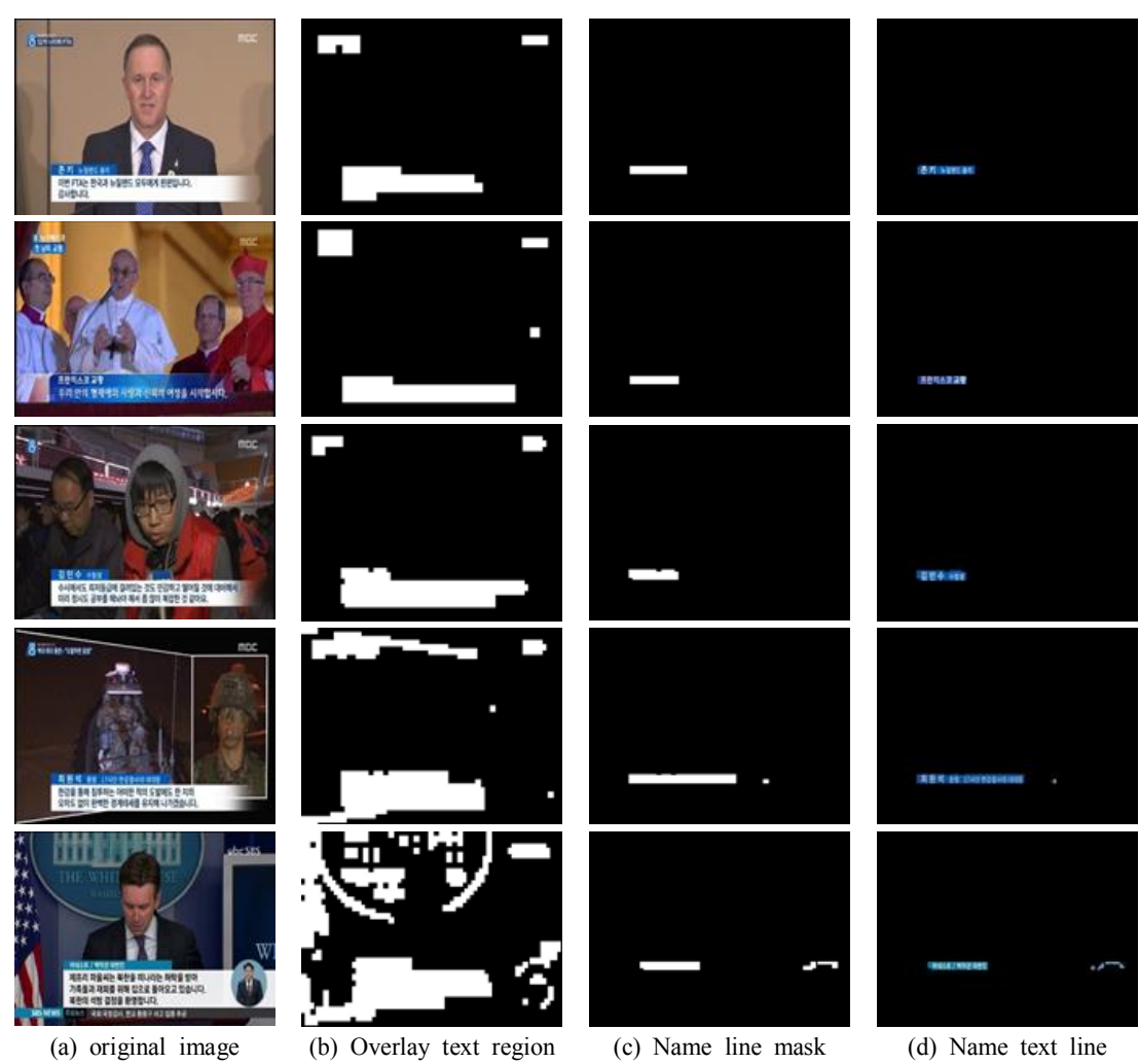
Fig. 6.5. The result of name text line detection and localization
