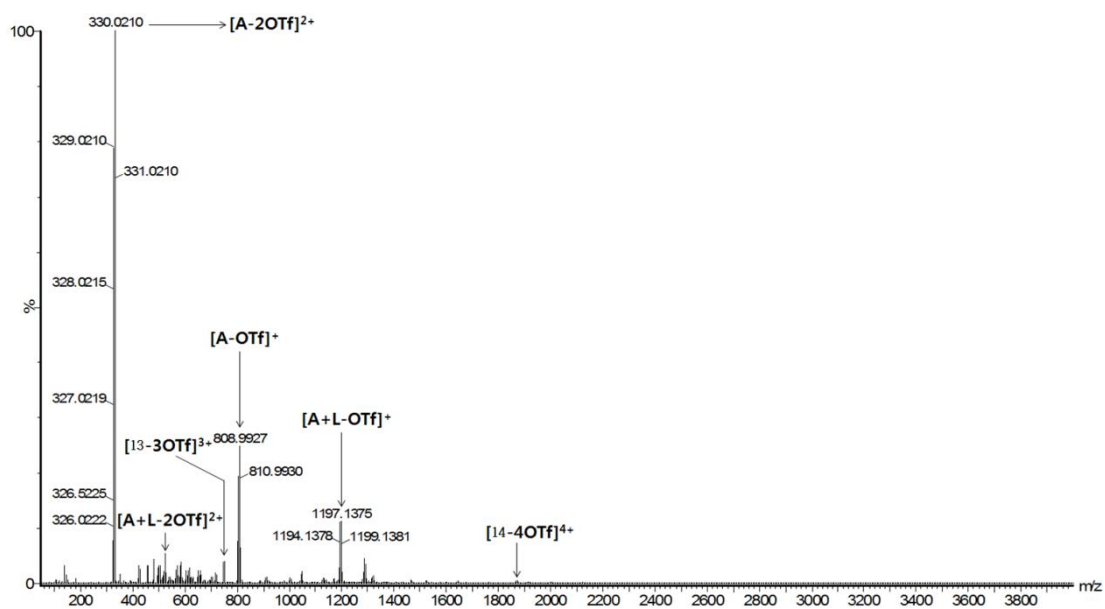
Figure 4.10 Full ESI mass spectrum of mixture 13+14 (Reaction in DMF [8.0 mM])
