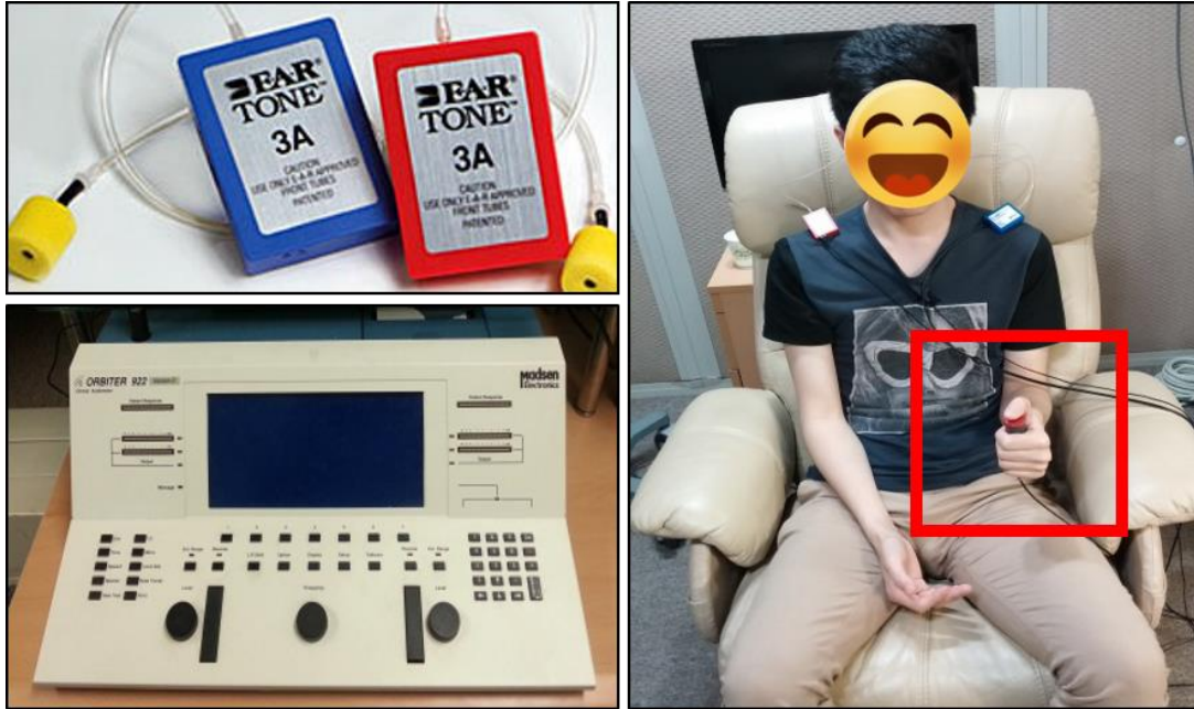
Figure 10. The equipment and environment for behavioral TEN test.
