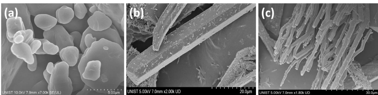
Figure 4-2. SEM images of (a) pure melamine, (b, c) supramolecular precursor after 24 h hydrothermal reaction time
