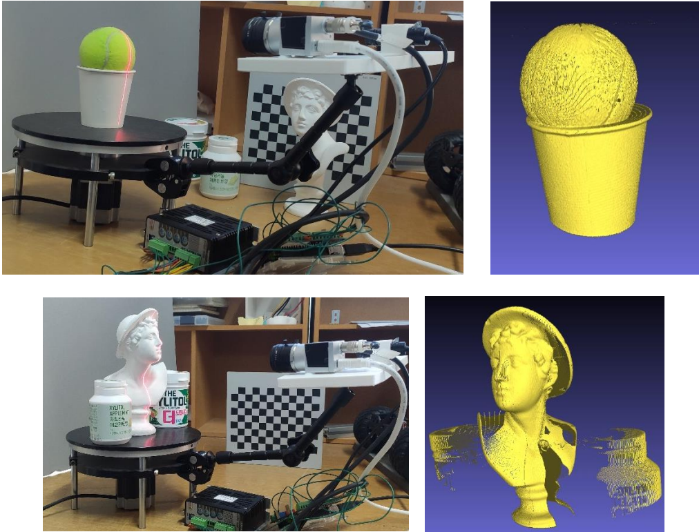
Figure 4.8. Scanning workspace for quality check and its scanning result.
