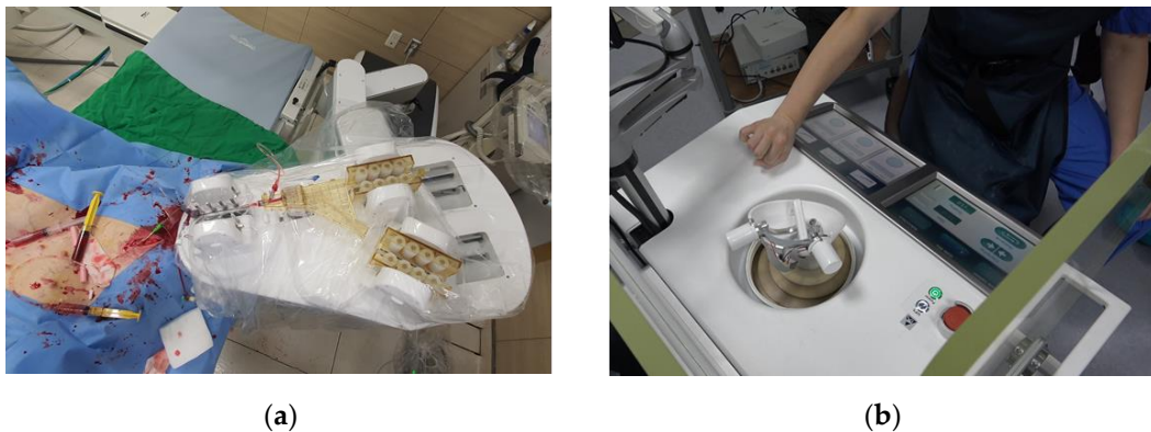
Figure 18. Setup of the animal experiment. (a) The slave robot beside the operation table and (b) the physician at the master console.
