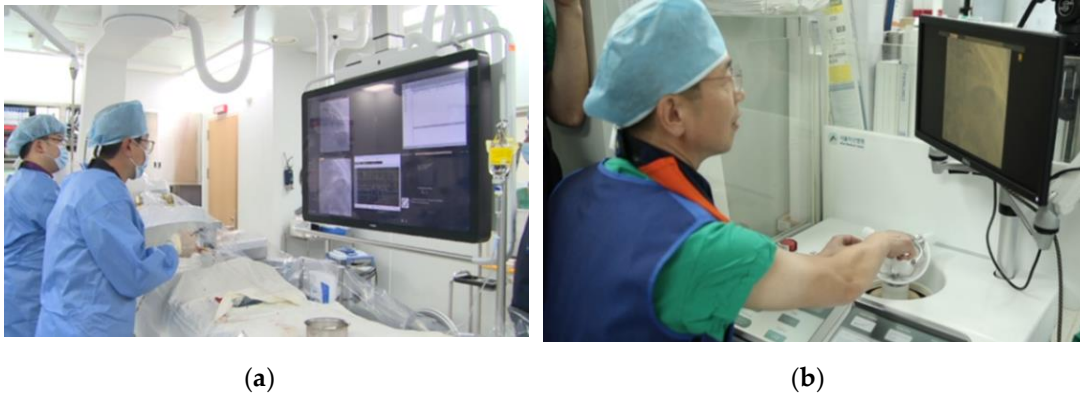
Figure 20. Setup of the clinical trial. (a) The slave robot and the patients in the operation room are shown. (b) The physician is located in the corner of the angiography room with the master console, behind a radiation-shielded glass wall.
